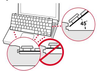
4. Pull down on the keyboard release tabs and then press down on the top portion of the keyboard. (Figure 11)
