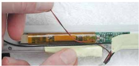
4. Warning: When removing the tape that bundles the reed switch cable assembly to the AirPort Card antenna cable, be careful not to strain or pinch the cables.
