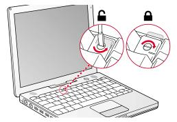
8. Release the keyboard by pulling down on the keyboard release tabs (located to the left of the F1 and F12 keys) (**Figure 3**), then lift the top portion of the keyboard up slightly, and toward the display.
