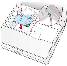
7. If you do not have an AirPort Card, flip down the wire holder over the AirPort Card antenna cable and secure it by inserting the prongs of the holder into the slots in the RAM shield. (Figure 11)
