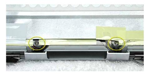
9. Peel up the tape that anchors the folded mesh strip of the LCD cable to the shield.
