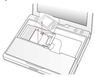
5. Lift the RAM shield out of the computer. Carefully pulling up on the wire holder may help to remove the shield. (Figure 8)
