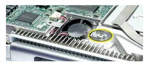
2. Lift the fan and bracket from the computer, and use a black stick to disconnect the connector from the logic board.
