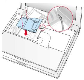
7. If you do not have an AirPort Card, flip down the wire holder over the AirPort Card antenna cable and secure it by inserting the prongs of the holder into the slots in the RAM shield. (Figure 13)
