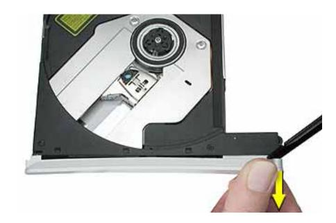
3. Use the flat end of the black stick to detach the middle tab and remove the door.
