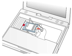
4. Use the wire holder to secure the AirPort Card in place by inserting its prongs into the slots in the RAM shield. (Figure 9)
