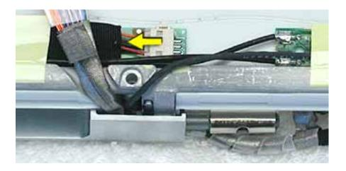
6. Remove the reed switch cable assembly.
