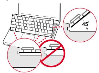
4. Pull down on the keyboard release tabs and then press down on the top portion of the keyboard. (Figure 14)
