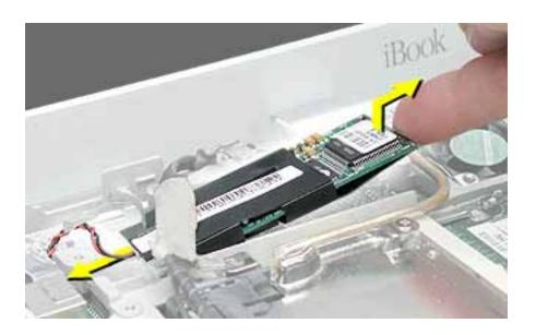
5. Install the replacement modem, and reassemble and test the computer.
