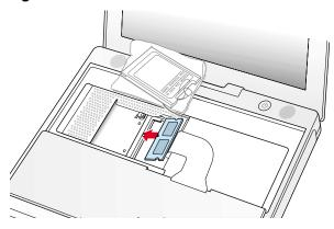
2. Gently push the top of the card down until the brackets snap onto both sides of the memory card to lock it into place. (Figure 11)
