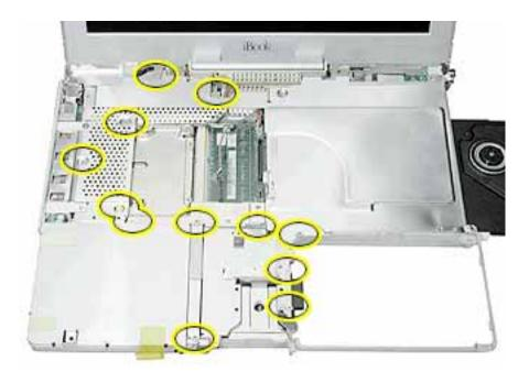
2. Using a black stick, carefully peel up, but do not remove, the foil strips and pieces of tape.
