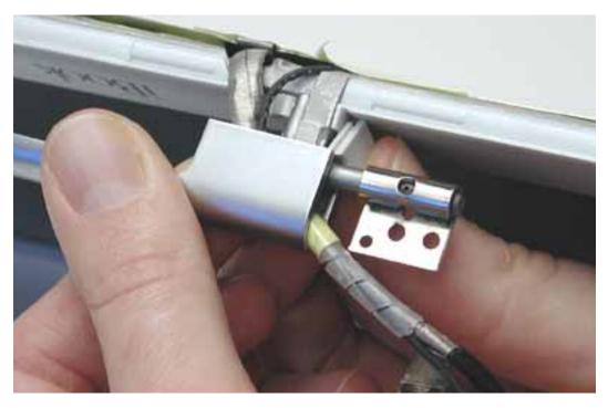
Make sure the clutch cap on each side of the clutch cover is firmly seated before installing the two screws.
