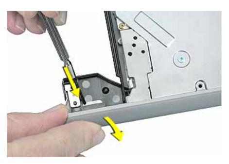
3. Release the tab at the other end of the door, and pull the door straight up to free it from the drive.
