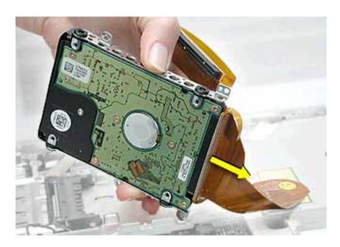
6. Holding the drive by the corners as shown, pull off the side rails (with grommets attached).
