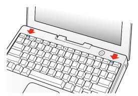
9. Flip the keyboard over and lay it on the palm rests and trackpad. (Figure 4)
